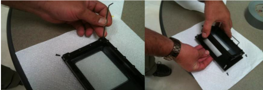
Figure 19: Remove PSA from basement
