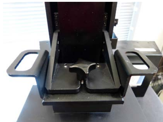
Figure 22: Mounted build platform
