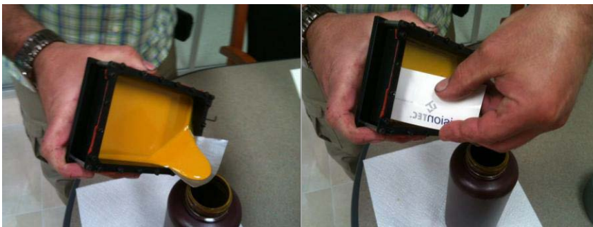
Figure 17: Remove material from basement
