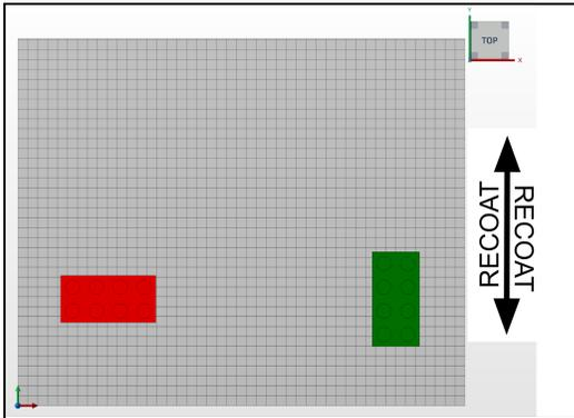
*The same part placed in two orientations on the Xtreme 8K: the left part does not face the movement of the recoater and is not recommended; the right part faces the movement of the recoater and is best practice*
