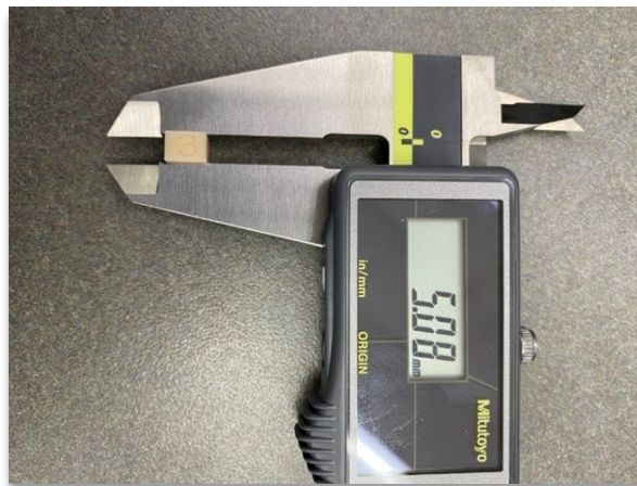
Figure 9. Calipers measuring calibration Cube 3.
