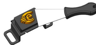
Figure 10: Separation of a model from the build platform
