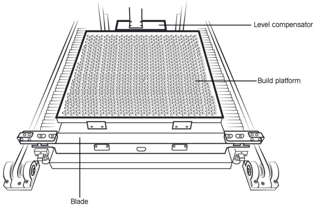
Figure 6: Upper printer compartment view (open)
