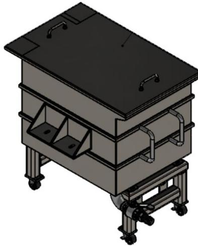
Figure 13: Material Tank and Drain Valve
