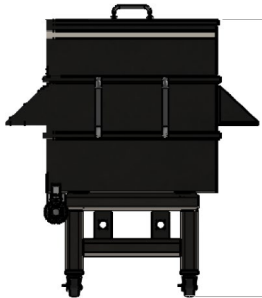
Fig. 8 Removable Material Vat Front View
